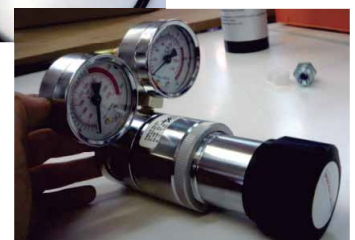
Detail of the pressure regulator of the H 2 bottle and hose
