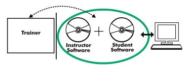
With no physical connection between trainer and computer (PC), this complete software package consists of an Instructor Software (INS/SOF) totally integrated with the Student Software (MINI-EESF/SOF). Both are interconnected so that the teacher knows at any moment what is the theoretical and practical knowledge of the students.
